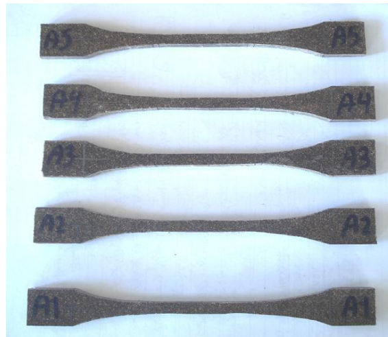
Fig. 8. Prepared tensile specimens.
