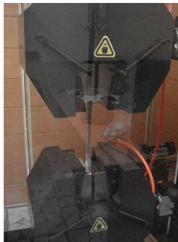
Fig. 9. Tensile strength test setup.
