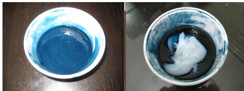
Fig. 4. Epoxy resin and hardener mixture.
