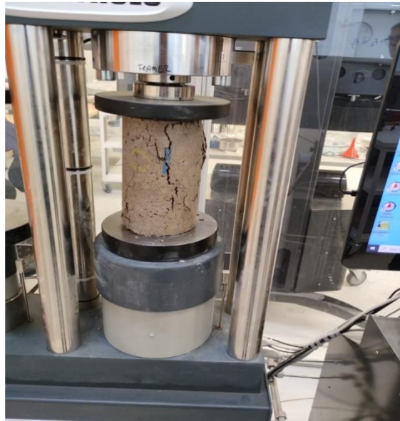
Fig. 7. A view of the compressive strength instrumentation and test.
