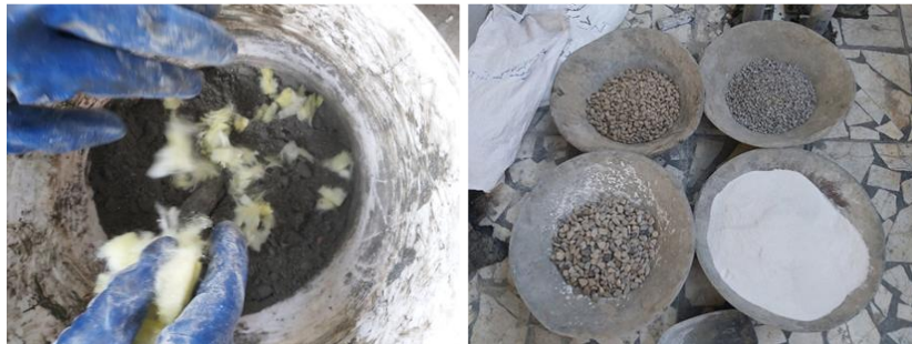
Fig. 2. Aggregate separation and incorporation of glass wool fibers.
