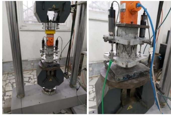
Fig. 3. Experimental setup for the compressive strength test.
