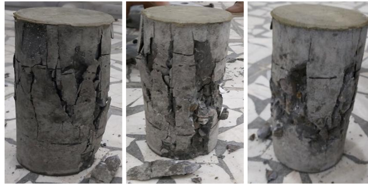
Fig. 4. Representative failure patterns of lightweight perlite concrete specimens under compression.
