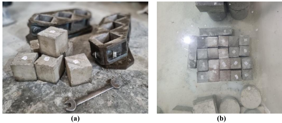
Fig. 3. Casting and curing of mortar specimens.
