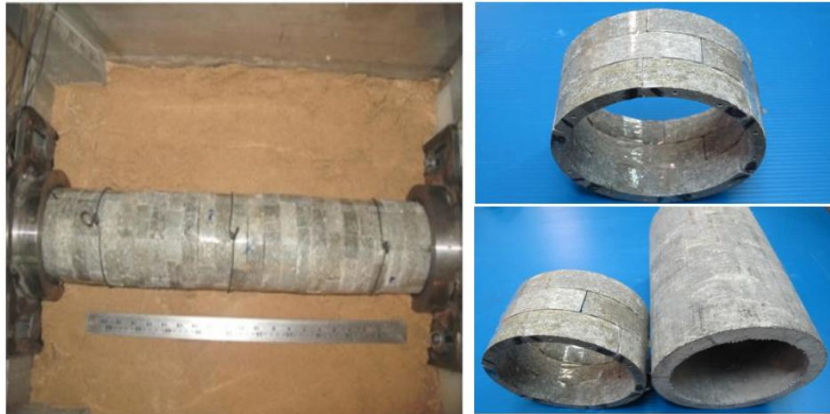
Fig. 1. Images of the construction process of the segmental tunnel using asbestos-cement pipe.
