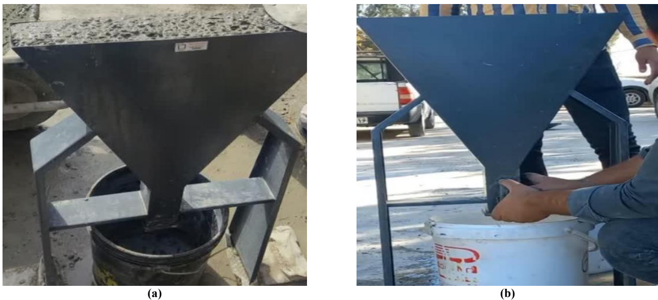
Fig. 7. The process of V-funnel test (a) Flattening the surface (b) Opening the valve.
