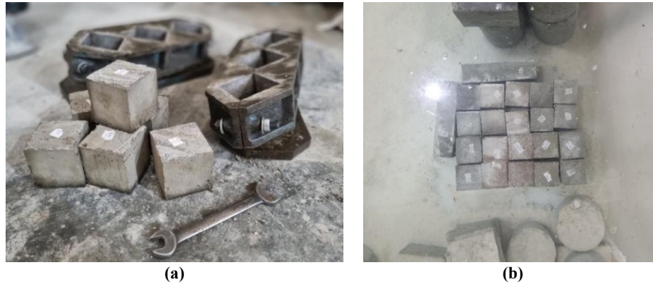
Fig. 3. Casting and curing of mortar specimens.
