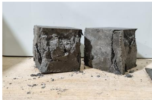
Fig. 7. Failure of mortar samples under compressive test.
