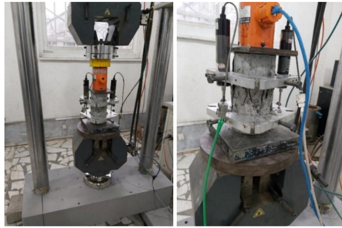
Fig. 3. Experimental setup for the compressive strength test.
