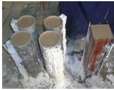
Fig. 5. Filled column formworks after placement and vibration.
