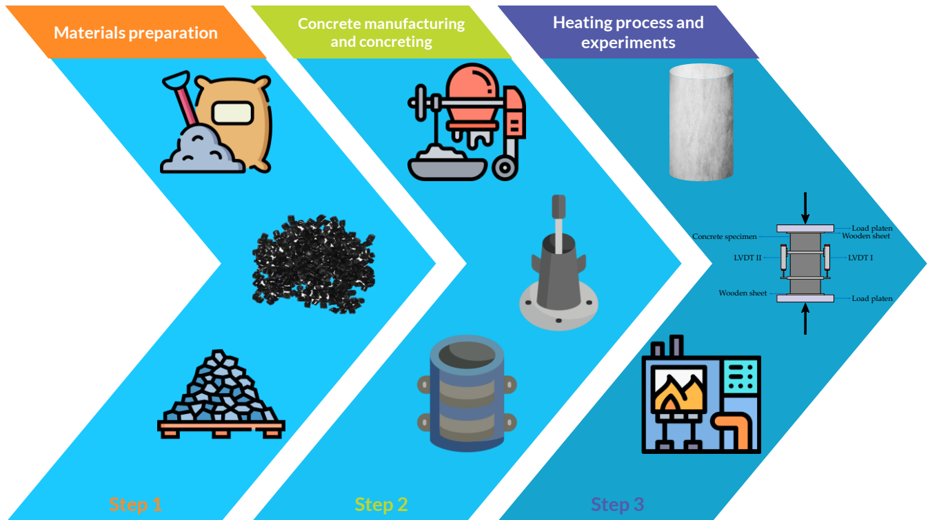
Fig. 7. High-strength nylon granule aggregate concrete manufacturing steps.
