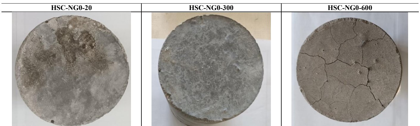
Fig. 36. HSC specimens containing NG after exposure to elevated temperatures.
