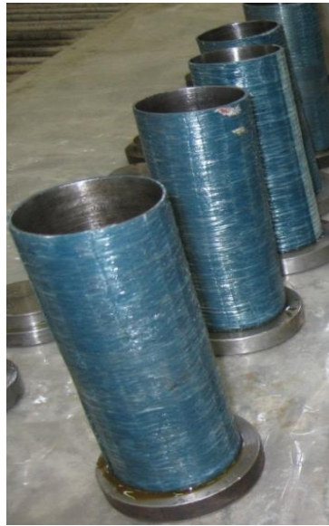
Fig. 2. Hybrid steel–FRP tube before concrete casting.
