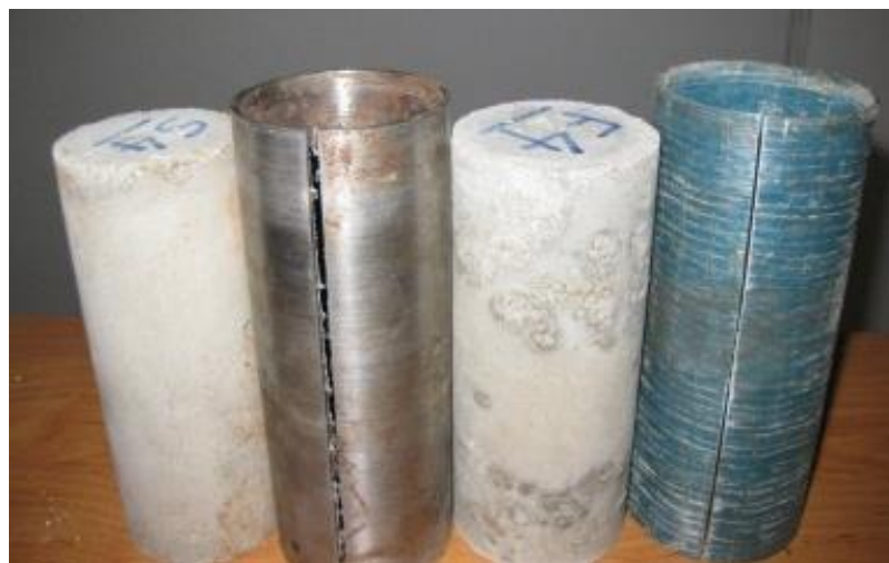
Fig. 4. Concrete cores extracted from confined specimens.
