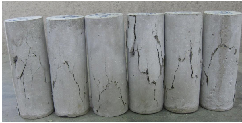
Fig. 7. Failure patterns of reference concrete specimens.
