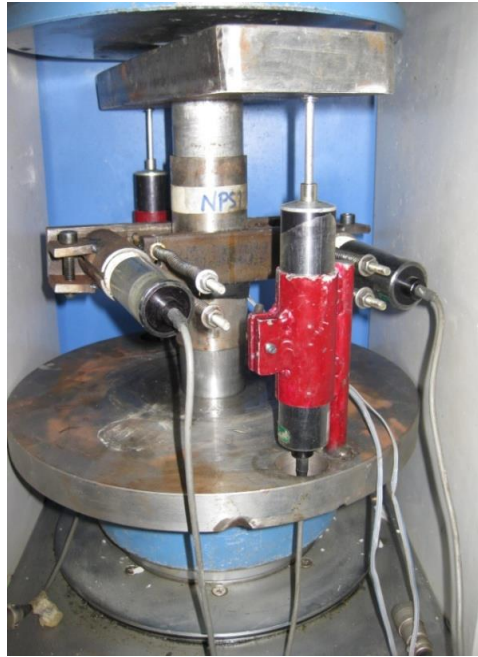
Fig. 5. A steel-confined specimen with instrumentation for loading and deformation measurement.
