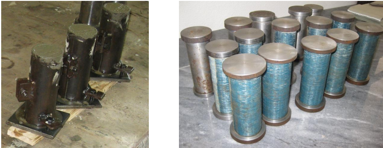
Fig. 3. (a) Control specimens (Group R), (b) Confined specimens with steel tubes (Group S), FRP jackets (Group F), and hybrid steel-FRP tubes (Group SF).
