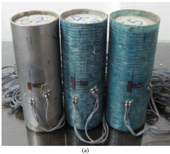
Fig. 6. (a) Strain gauge arrangement on confined specimens, (b) Loading setup for confined specimens.
