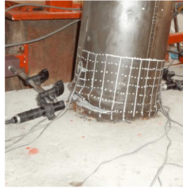
Fig. 7. Comparison of experimental and simulated damage states (cracking, yielding, and buckling) at incremental drift ratios: (a) 2%, (b) 4%, (c) 6%, (d) 8%.
