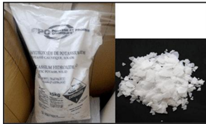
Fig. 4. Potassium hydroxide (KOH) flakes used as the alkaline activator in the geopolymer concrete formulation.
