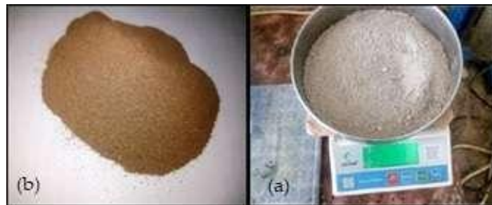
Fig. 2. Photographs of the (a) blast-furnace slag, and (b) ceramic powder used in the geopolymer concrete mixtures.
