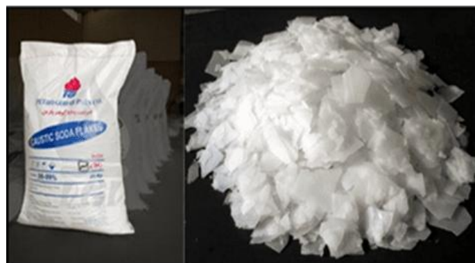
Fig. 3. Sodium hydroxide (NaOH) flakes used as the alkaline activator in the geopolymer concrete formulation.
