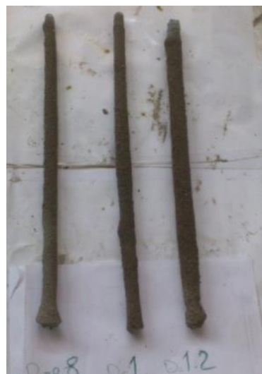
Fig. 4. Micropile specimens retrieved after bearing capacity testing.
