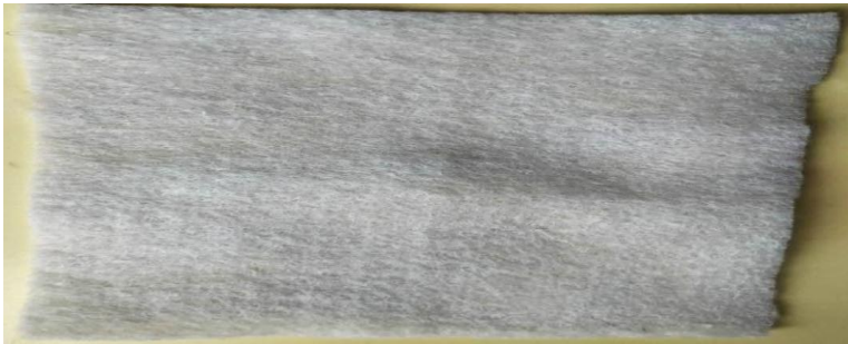
Fig. 2. Enclosing geotextile used in the stone columns.
