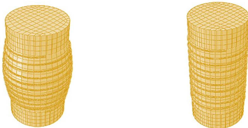
Fig. 5. Final finite element model and deformed configuration.
