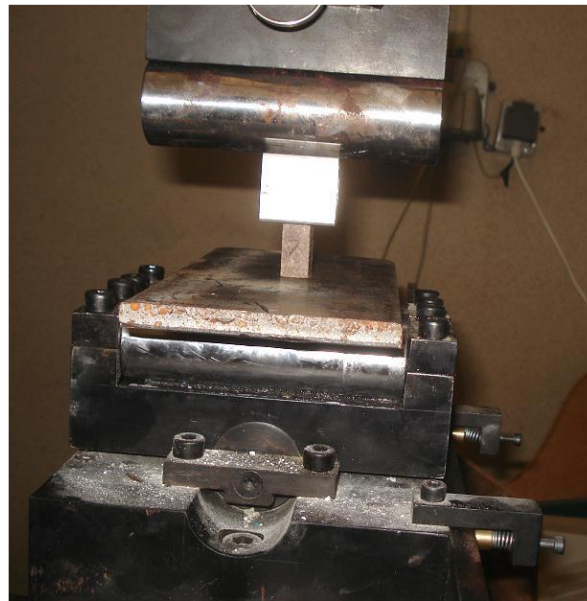
Fig. 6. Compressive strength test setup.
