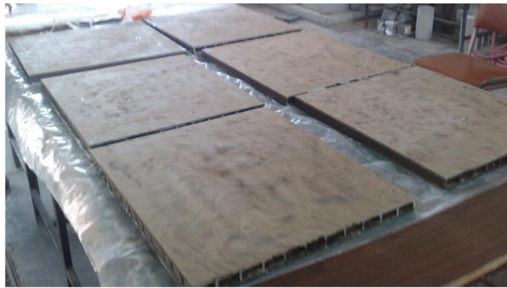
Fig. 10. WPC surface after glaze removal.
